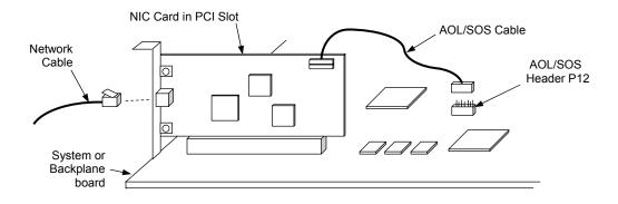
Figure 5-15. Remote System Alert Implementation (Generic Representation)
